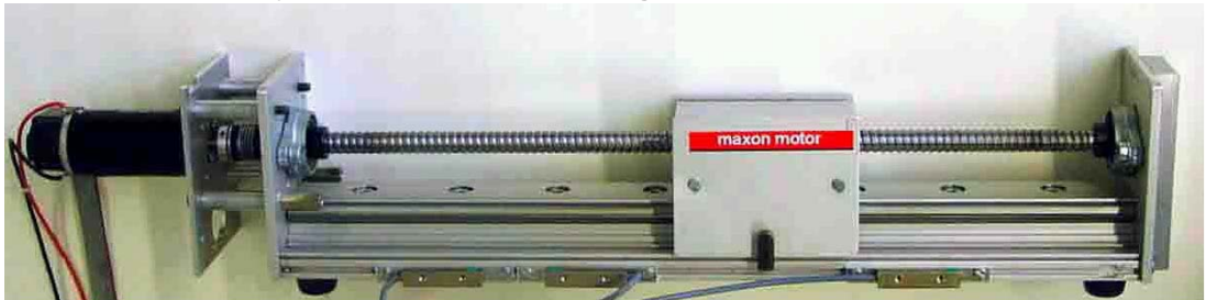
Figure 9-94 Controller Architecture – Example 2: System with low Inertia/high Friction
