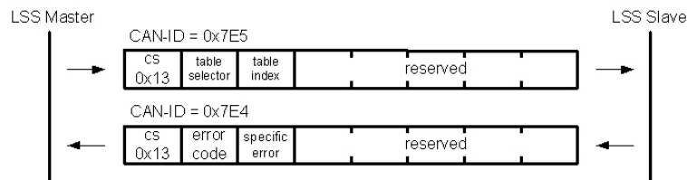
Figure 7-63 LSS – Configure Bit Timing Parameters
